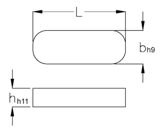
$\begin{array}{ll} b & = 4 \\ h & = 4 \\ L & = 18.0 \\ Tolerance \ b = 0.030 \\ Tolerance \ h = 0.075 \end{array}$
